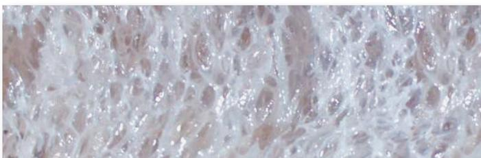
A “water fearing” material. Hydrophobic grouts have little to no affinity for water. As they cure, they repel water and push it back into the substrate.
