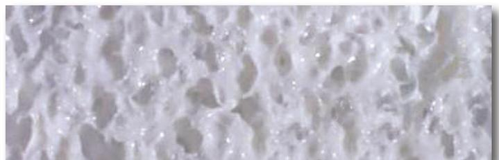
A “water loving” material. Hydrophilic grouts thrive on water and seek it out within the crack and all the tributaries and fissures associated with it. As they cure, they absorb water, replacing it in the substrate.
