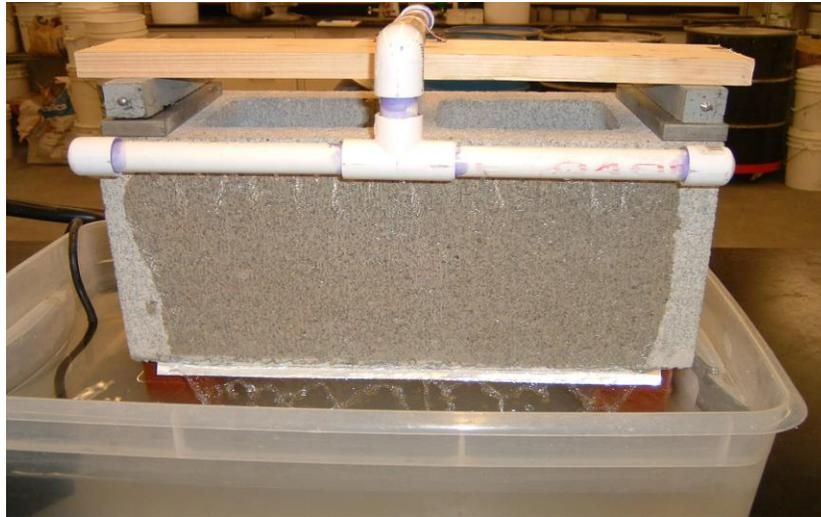
***Method:*** - Prior to testing, store units in laboratory air (24+/- 8°C [75+/- 15°F]) with a relative humidity of less than 80% for not less than 48 hours. Units shall have no visible moisture prior to start of testing.
