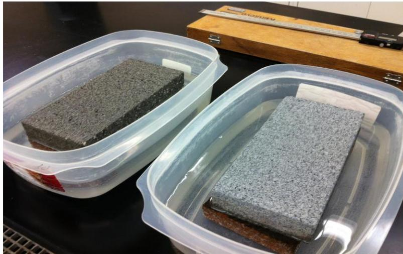
***Method:*** - Prepare the sample by saw cutting the face shell from CMU keeping the web “tabs” as short as possible without damaging the back of the face shell.
