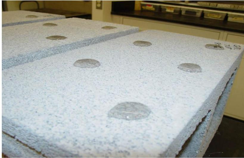
***Method:*** - Three full-sized masonry units are tested from each test mix submitted. Units shall have no dust or visible moisture on the surface.
