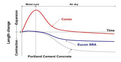
The graph on the left shows the shrinkage typically experienced in reference Portland cement based concrete and concrete utilizing *Shrinkage Reducing admixtures* and *Shrinkage Compensating materials*.
