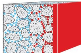
VANDEX SUPER is applied and a crystalline growth occurs within the capillaries, thus eliminating the pathways for water.
