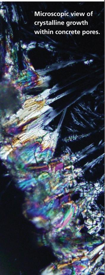
Microscopic view of crystalline growth within concrete pores.
