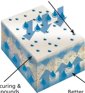
High solids curing & sealing compounds can offer greater film thickness for added protection
