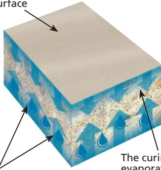
Moisture held within the concrete ensures proper hydration of the cement
