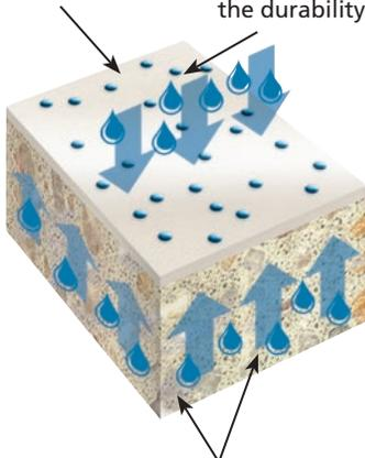
Sealing products are specifically designed to repel liquids. This results in improved chemical and moisture resistance, and improves the durability of the concrete.
